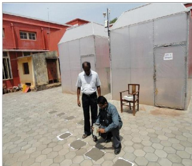
Plate A : Recording spectral reflectance of black soils of CRS, Veppanthattai at 11.00 am to 12.30 pm
