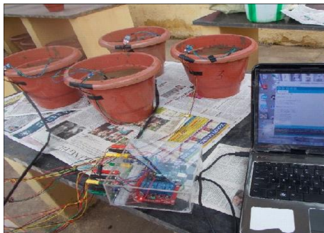
Plate C : Performance of soil moisture sensor in black soil
