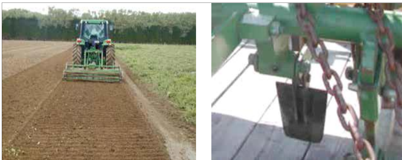
Fig 1 and 2 : Powered tillage tools used with horticultural crops: rotary tiller (left), and spader (right)
