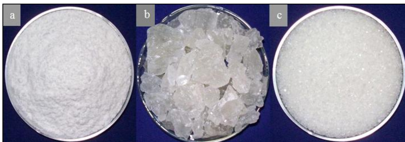
Fig. 1 : Different sources of carbon: (a) AR grade sucrose; (b) Rock sugar; (c) Common grade sugar
