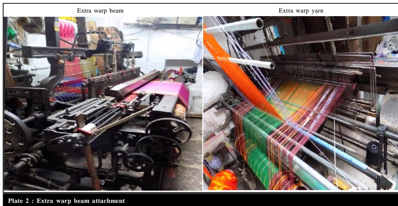
Plate 2 : Extra warp beam attachment
