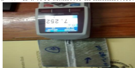
(b) Measurement of surface roughness by Mitutoyo Talysurf
