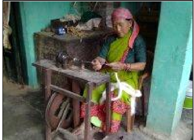
Plate 12 : Spinning of nettle yarn on Bageshwari charkha
