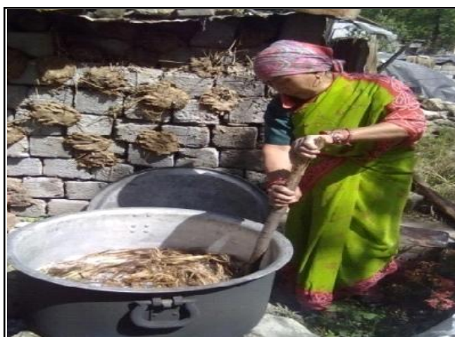
Plate 5 : Degumming of nettle fibres
