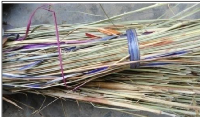
Plate 1 : Kanss grass (core material)
