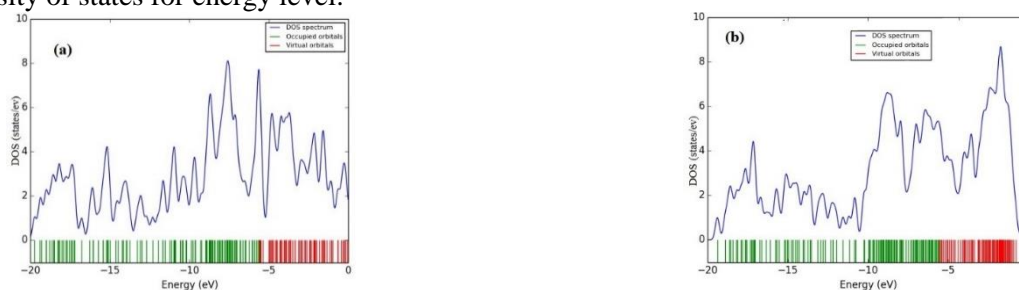
Figure.2. DOS of pristine PNRs: (a) Black and (b) Blue. DOS spectrum (blue line), occupied orbitals (green line) and virtual orbitals (red line).
