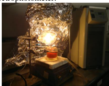
Figure.2. Main parts of the photocatalytic cell used in Photocatalytic degradation of malachite green dye
