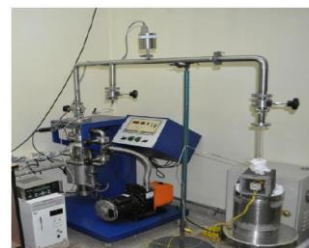
Figure.2. Sievert's apparatus setup for gaseous hydrogen charging
