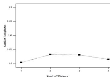
**Figure.6. Surface Roughness Vs SOD**
