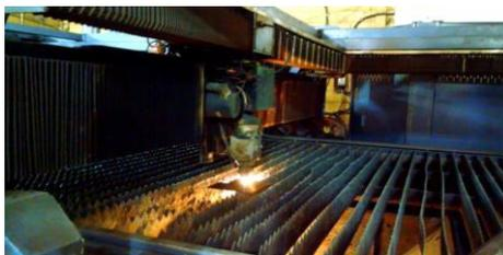
**Figure.2. Truflow 4000 CO<sub>2</sub> Laser cutting Machine**
