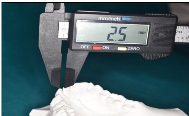
Figure 6: Digital vernier caliper to measure little's irregularity index on study models.
