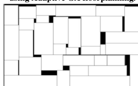
Figure.8. Floorplan of ami33 benchmark with area = 1.21mm 2 and total Interconnect length = 31.33mm
