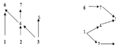
Figure.2. (a). Non slicing floorplan Vertical and Horizontal Constraint graph
