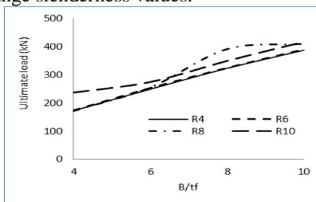
**Figure.7. Plot between Ultimate load versus flange slenderness**
