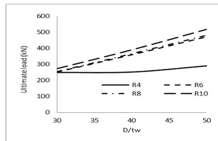
**Figure.9. Plot between Ultimate Load versus web slenderness**
