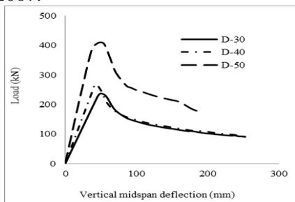
**Figure.8. Plot between Load versus deflection – varying web slenderness**
