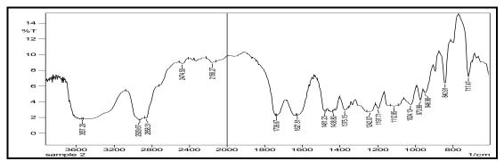
Fig 4: FTIR spectrum of Soluplus
