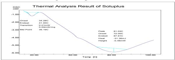
Fig 9: DSC Thermogram of Soluplus
