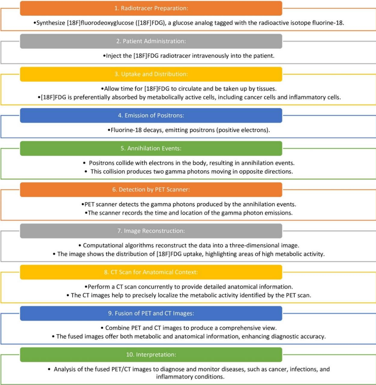
Figure 2: Mechanism of PET CT Scan
