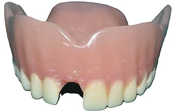
Figure 3: Debonding of denture tooth.
