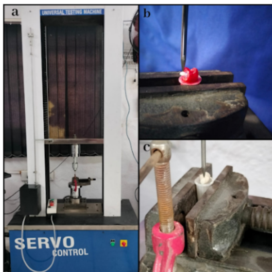
Figure 2: a: Universal testing machine; b,c: Tooth mounted with chisel-rod at dentin-resin interface on the universal testing machine
