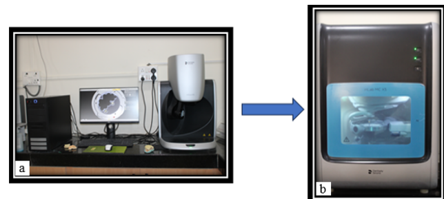
Figure 2: a: Metal die scan with extraoral scanner (Dentsply Sirona); b: Milling machine (In lab MC X5).
