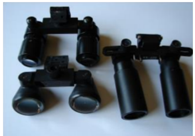
Fig. 5: A 2.5x Galileian binocular loupe (lower left), and a 4x (top left) and a 6x (right) Keplerian binocular loupe shows the longer barrel length for higher magnification Keplerian binocular loupes, and the wider diameter objective lens of the Galileian binocular loupes.
