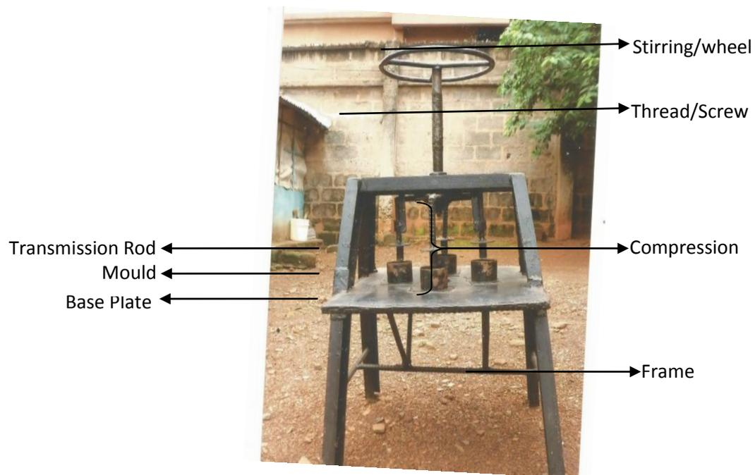
Plate 1.0: The fabricated screw press.
