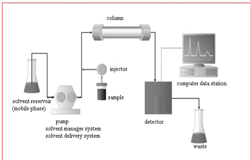
Fig.1: Components of HPLC instrument block diagram.
