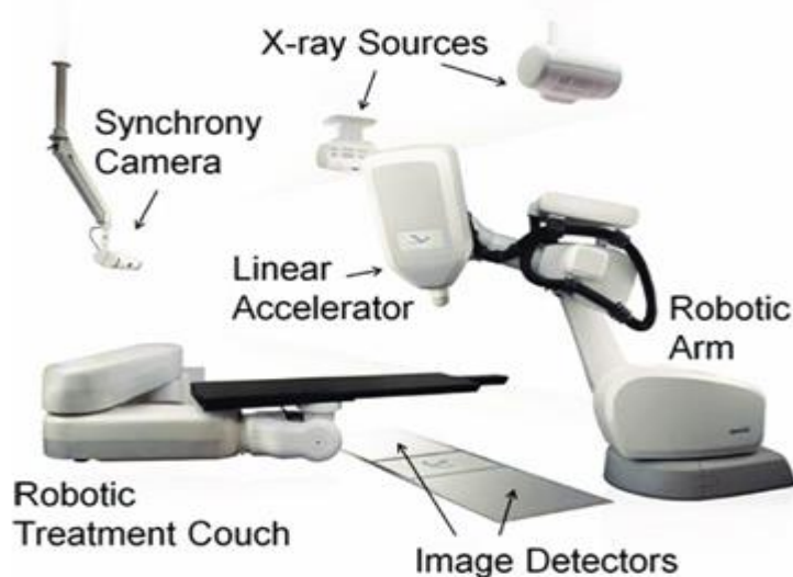
Figure 1. CyberKnife setup parts. A six-jointed robotic arm carries a small linear accelerator and may freely move around the patient. Nearly "real-time" target imaging is achieved by positioning two kilovoltage x-ray sources orthogonally. Using light-emitting diodes attached to the patient's chest, the infrared Synchrony camera can track the patient's chest wall's movement.
