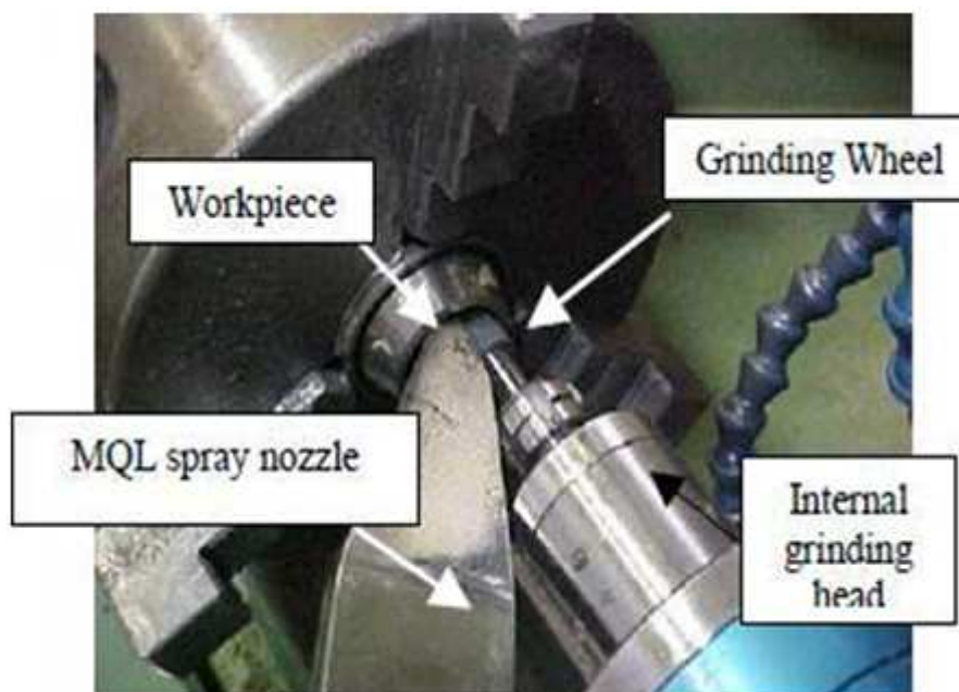
Figure 2. Position of the MQL Spray Nozzle in the Cutting Region
