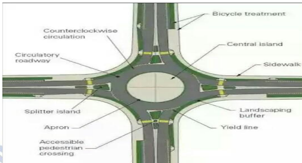
Fig 1.2 parameters of roundabout
