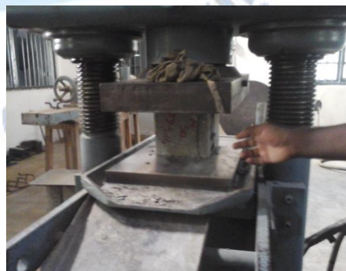
Fig1: compressive strength test of cube
