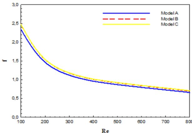
Figure 7: Variation of pressure loss coefficient with Reynolds number
