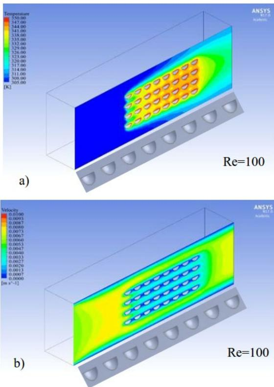
Figure 11: Temperature and velocity contours for Model A
