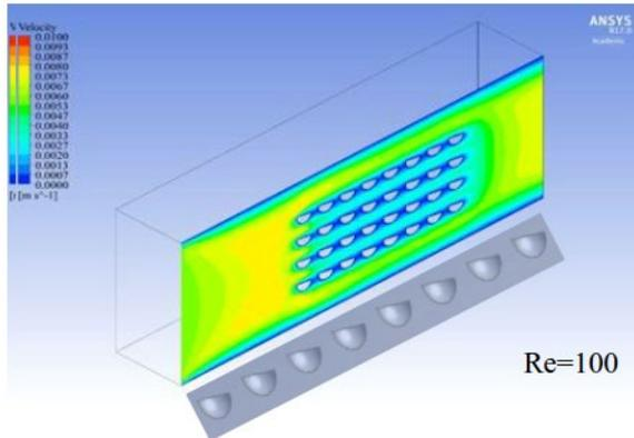
Figure 12: Temperature and velocity contours for Model B
