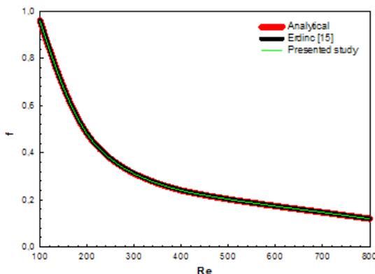
Figure 5: Comparing the results obtained for *f*-friction factor
