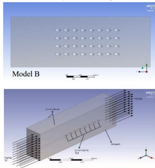
Figure 2: Boundary conditions used in numerical calculations
