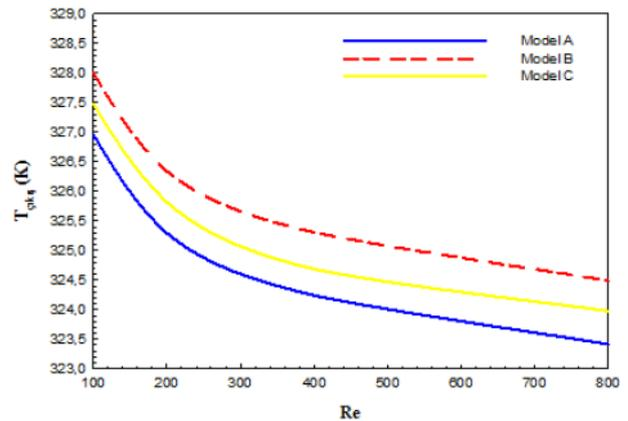
Figure 8: Variation of fluid outlet temperature with Reynolds number
