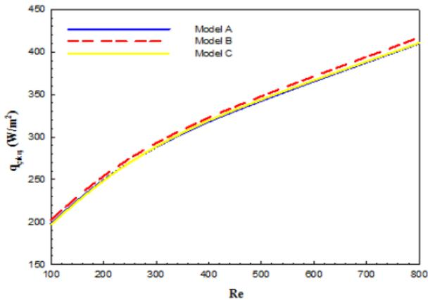
Figure 10: Variation of heat flux with Reynolds number in the outlet
