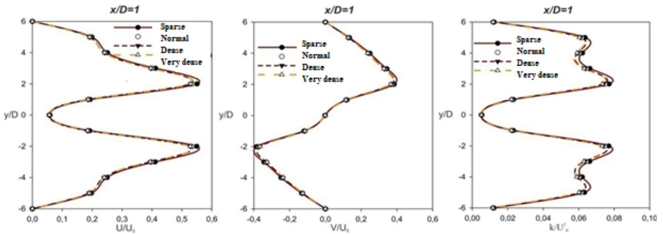
Figure 3: Variation of x, y velocity component and turbulence kinetic energy according to different mesh numbers respectively, Re = 100
