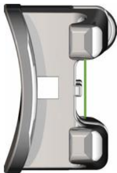
Fig 6: Slot height of a bracket
