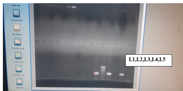
Fig. 3: Photograph of amplified bla IMP gene in P. aeruginosa ; the amplified DNA band size was obtained 256bp, Lane 1 and L 3 is the sample positive for bla IMP ; L2 corresponding to 100bp ladder used; L4 corresponds to the negative control and L5 corresponds to the positive control
