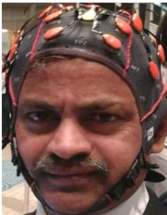
Fig. 2: A wireless head worn electrode system
