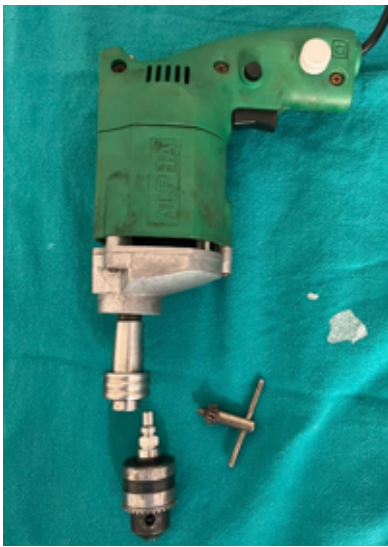
Fig. 1: Drill with detachable chuck, speed controller, and cannulated system
