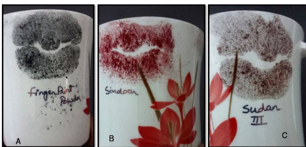
Fig. 2: (a): Lip print developed by fingerprint powder on bone china; (b): Lip print developed by vermilion on bone china; (c): Lip print developed by Sudan III on bone china
