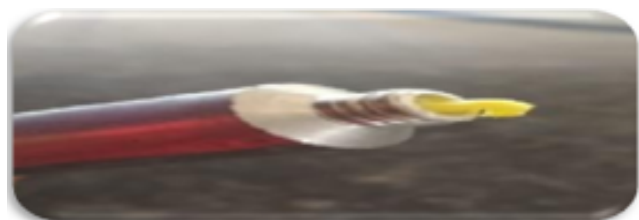
Fig. 7: Extrudability test for ointment
