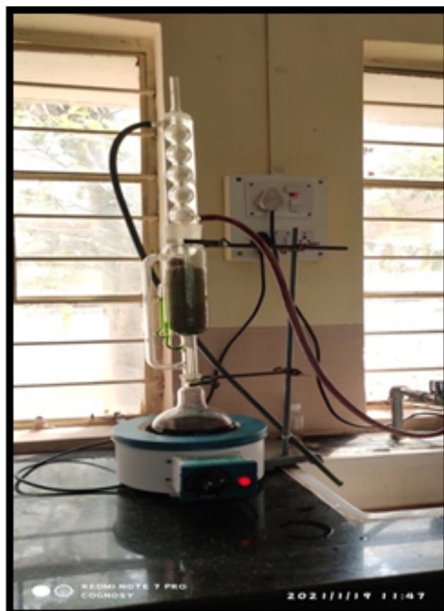
Fig. 2: Soxhlet apparatus during extraction process
