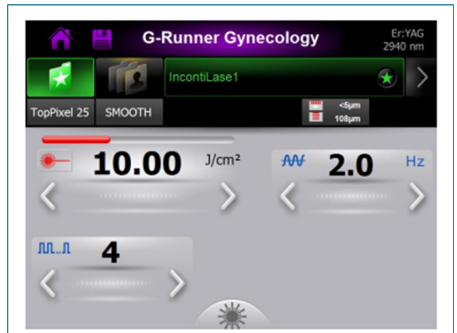
Fig. 15: Application screen for the G-runner IncontiLase1 treatment showing a burst of four SMOOTH pulses per each position
