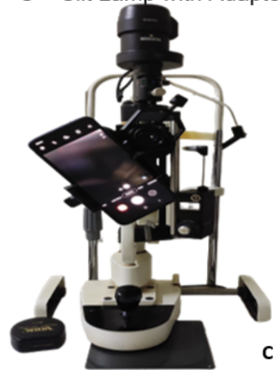
Fig. 4: Showing the telescope adaptor used in study as well as its attachment with eye piece of slit-lamp bio-microscope (available in all online shopping Platforms)
