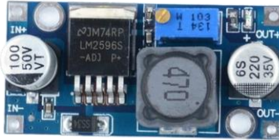
Figure 14. Buck Converter used for step down voltage output [12]
