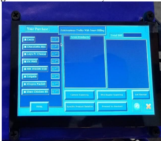
Figure 7: Autonomous Trolley Billing Detail with Touch Screen LCD
