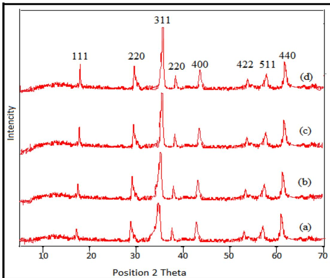
**Fig. 1:** X-ray diffraction patterns for (a) CuFe<sub>2</sub>O<sub>4</sub> (b) 1% Ag doped CuFe<sub>2</sub>O<sub>4</sub> (c) 2% Ag doped CuFe<sub>2</sub>O<sub>4</sub> (d) 3% Ag doped CuFe<sub>2</sub>O<sub>4</sub> powders annealed at 350 °C
