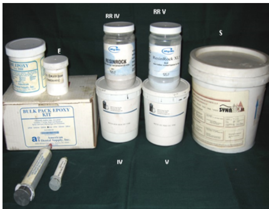
Fig. 2: Photograph showing the materials tested in this study. Clockwise from L - R: E - Epoxy resin, RR IV – Resin modified type IV gypsum, RR V – Resin modified type V gypsum, S – Synthetic gypsum, V – Type V gypsum, IV – Type IV gypsum.
