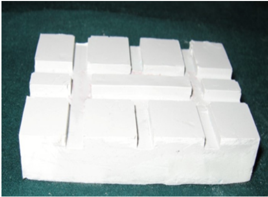
Fig. 1: Photograph showing the master die for fine detail reproduction
