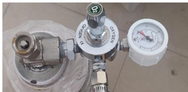
**Fig. 1:** FA valve with a flow meter that can be directly connected to a patient.
