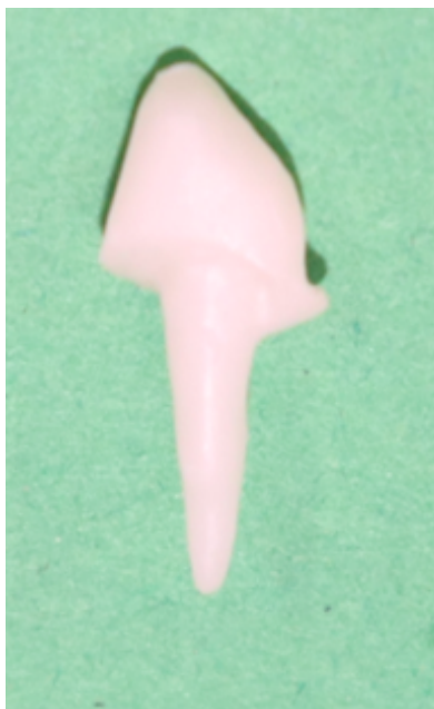
Fig. 5: Custom post, Sintered and finished Zirconia post
