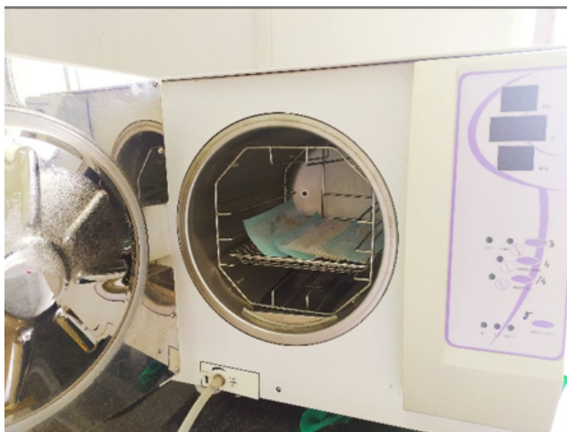
Fig. 3: Autoclave pouches with instruments placed inside the autoclave machine and autoclaved at 121°C under 15 psi for 15 minutes
