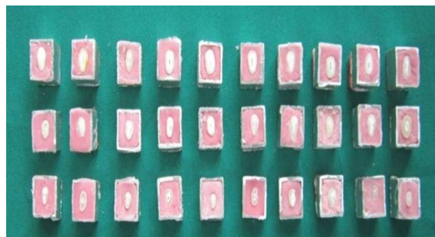
Fig. 1: Dentin samples mounted in self curing acrylic resin.
