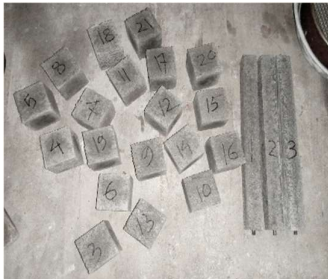
Figure 1: Preparation of mortar specimens
