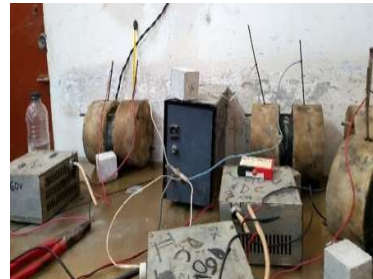
Figure 3: RCPT test setup of cylindrical specimen
