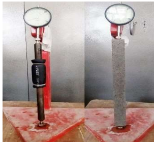
Figure 2: Length measurement of bar specimen
