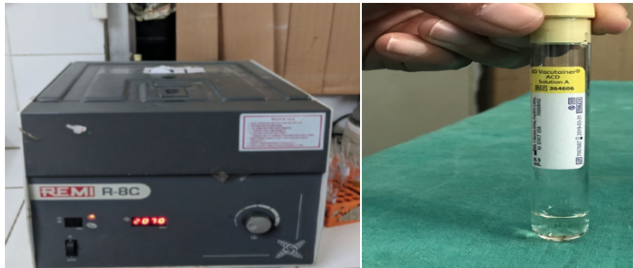
Fig. 1: a: Centrifugation machine. b: Showing PRP tube containing Acid Citrate Dextrose (ACD Tube)
