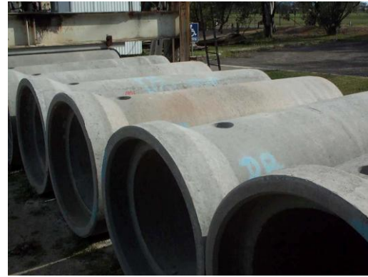
Figure 1: Geopolymer Concrete 1500 mm Sewer Pipes (3, 4)
