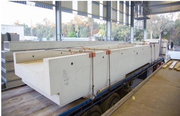
Figure 3: Precast Geopolymer Floor Beams (19, 20)
