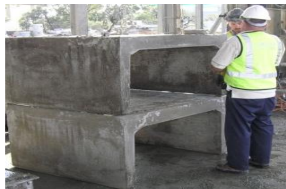
Figure 2: Precast Geopolymer Box Culverts (12, 18)
