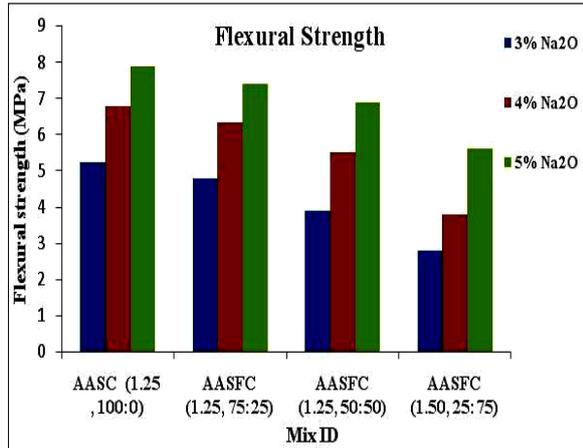
Fig. 5 Flexural strength of mixes for different activator modulus at various Na<sub>2</sub>O dosages
