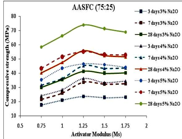
Fig. 2 Strength of AASFC (75:25) mixes for different activator modulus at various Na<sub>2</sub>O dosages
