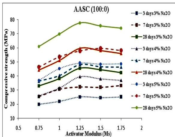
Fig. 1 Strength of AASC (100:0) mixes for different activator modulus at various Na<sub>2</sub>O dosages
