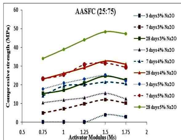
Fig. 4 Strength of AASFC (25:75) mixes for different activator modulus at various Na<sub>2</sub>O dosages
