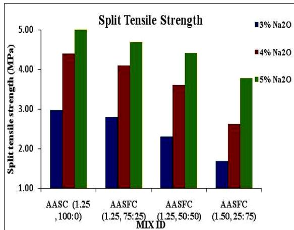
Fig. 6 Split tensile strength of mixes for different activator modulus at various Na<sub>2</sub>O dosages
