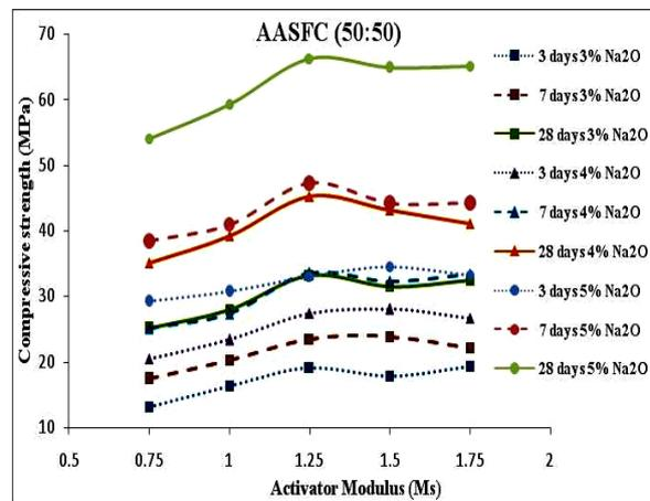
Fig. 3 Strength of AASFC (50:50) mixes for different activator modulus at various Na<sub>2</sub>O dosages
