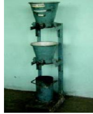
Fig: 2 Compaction Factor test
