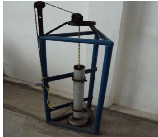
Fig 3 Test Set Up For Impact Strength
